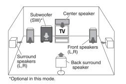
Although only Dolby Digital soundtracks incorporate a separate low frequency channel, connecting a subwoofer will also improve deep bass performance in the other surround modes. The indication **"LFE**" appears in the display when a signal is being
